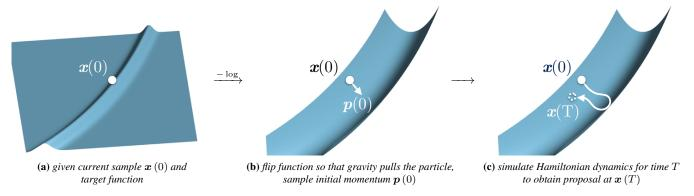
Figure 3: HAMILTONIAN MONTE CARLO: Given the current sample position  $\mathbf{x}(0)$  and a target function (the 2D slice from Figure 2), a physical analogy of Hamiltonian Monte Carlo is: (a) first it takes the logarithm of the target function and flips it upside down so that "gravity" pulls towards high contribution areas. (b) Then it gives the current sample an initial momentum  $\mathbf{p}(0)$  and (c) lets the point move for some time T with respect to the geometry of the flipped function.
