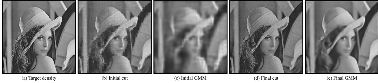
Figure 3: As a simple two-dimensional application of our method, we fit a 1024-term GMM to an image-based target density function (a). Our method starts with a coarse initial cut (b) and GMM parameters (c) and refines them until convergence (d and e).
